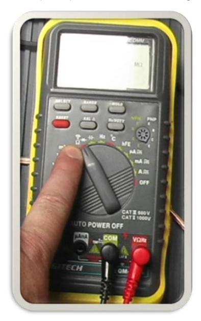
Connect the multi-meter leads to the terminals in the RJ11 connector as shown in the next image. The reading should show an overload or open circuit.
