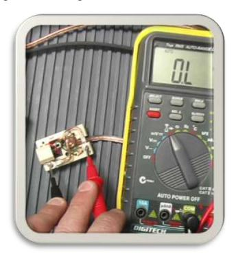
When someone stands on the mat the tone should sound or the meter should read a low resistance measurement close to zero.
