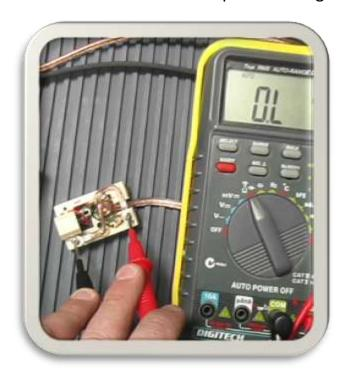
If this fails to work unscrew the cable and hold the multi-meter leads to the ends of the cable and repeat the test. If this fails there is a broken wire in the cable or mat and the unit needs to be replaced.
