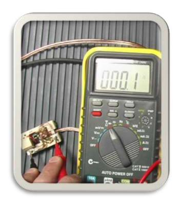
When they step off the mat the tone should stop and the resistance reading should show an overload or open circuit again.
