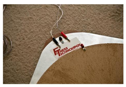
Plug the red banana plug into the red socket and the black banana plug into the black socket (see below).
