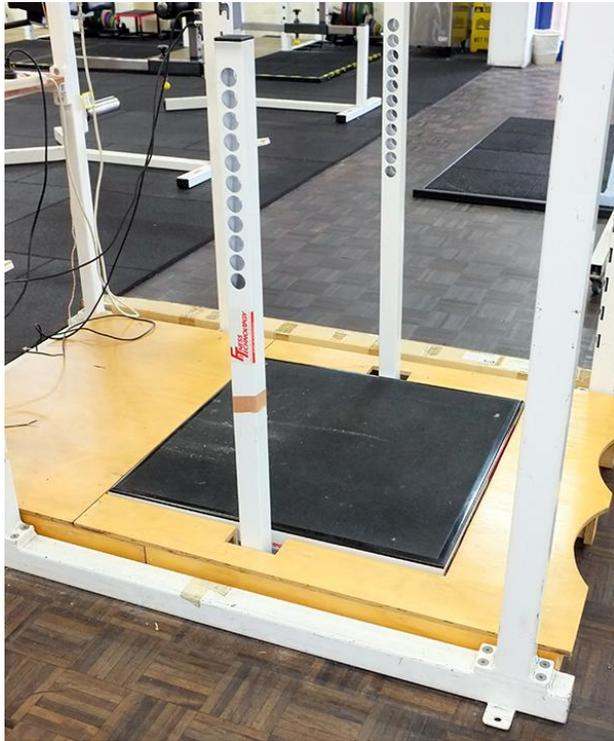
Then the Extension poles can be inserted in the uprights when testing for Isometric Squat or Calf raise is required.
