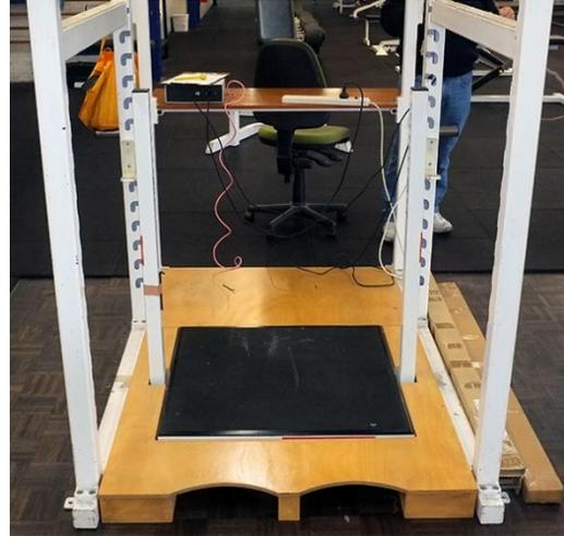
To Install the MTP Rig in the FT700 Power cage you start by installing the rectangular plywood half of the of the Force plate surround in the rear of the power cage as shown below. Then place the MTP rig base up against the surround. The force plate can then be moved into position and the USB and Cat5e cables run through the hole of the plywood surround
