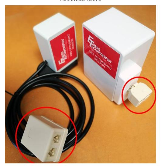
The new sensor still requires no reflector greatly reducing setup times. It also has a range compatible with the old version (2 metres in front of sensor) and can used in conjunction with the old sensor. More information is available on the KMS page of our website (Here).
