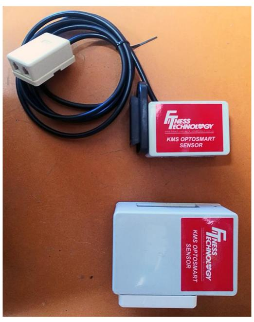
It also has a lead with a double RJ11 socket that removes the need for the double adaptor used in the old sensor version.
