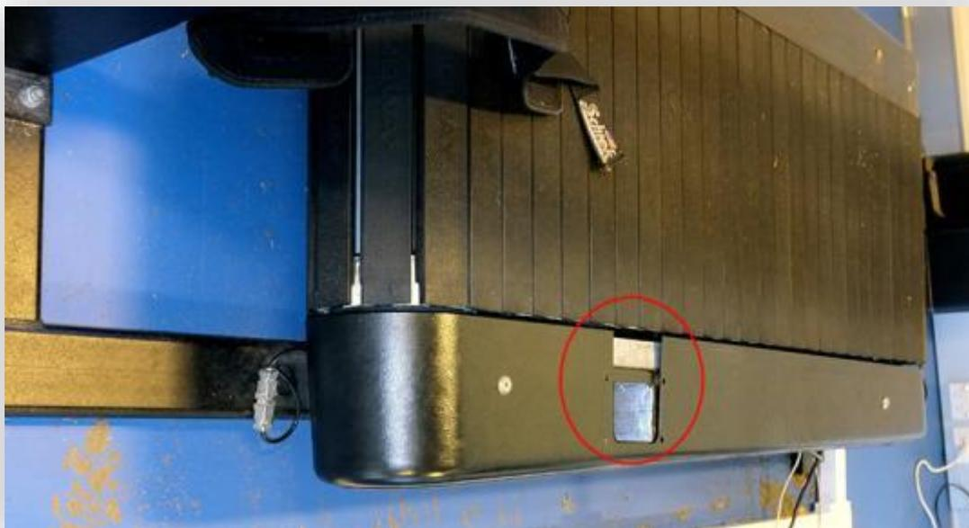
Once all screws are removed you can slide the side panel off. This will give you access Printed circuit board (PCB).
