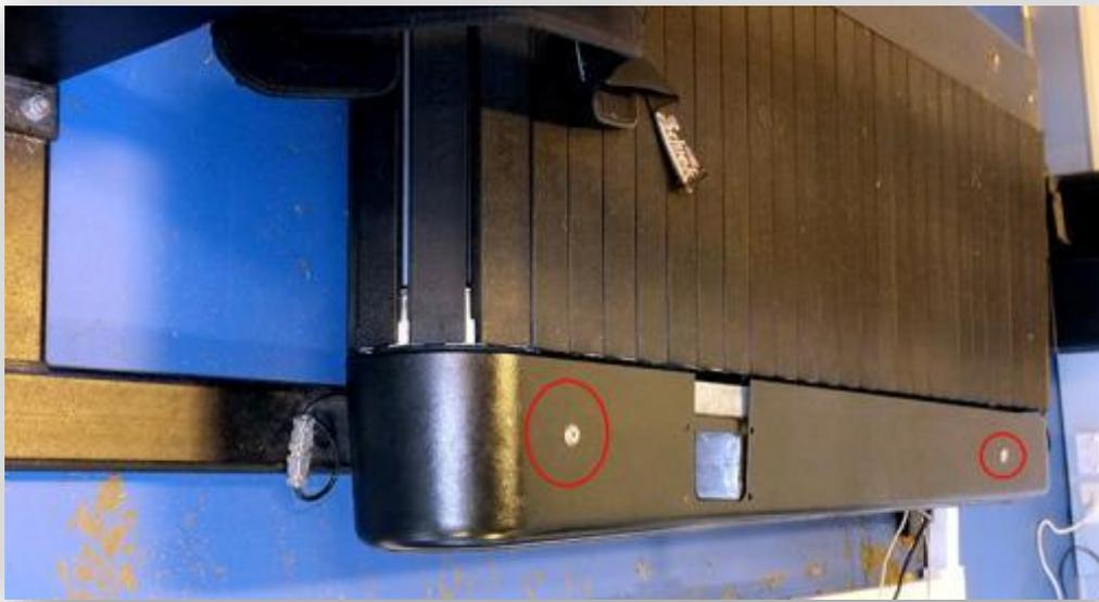
If the Upright for the control panel is still connected you will also need to remove the three screws that hold the panel that surrounds the upright.
