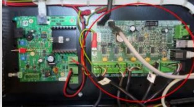
**Make sure to Turn off and unplug the power at the wall before touching anything inside the treadmill.** Start by unplugging the USB lead (see below)
