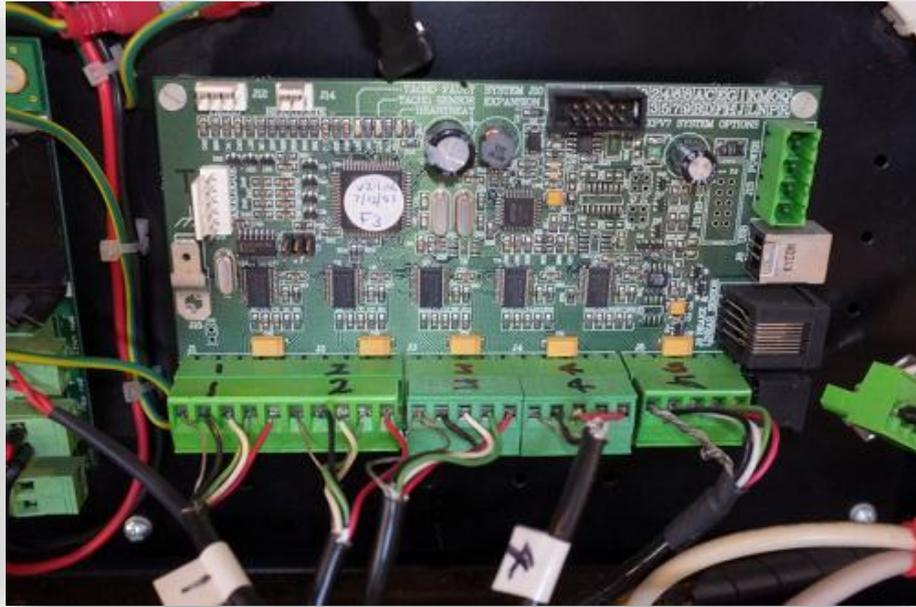
Now you can unplug the load cells from the PCB. **Do this by pulling on the connector not the cable.**
