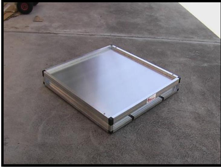
The carry case is made from fabricated Aluminium RHS frame with 1mm thick Aluminium sheets on the base & top.
